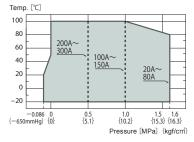
. Use after confirmation that maximum operation pressure and maximum service temperature is within the operation range
